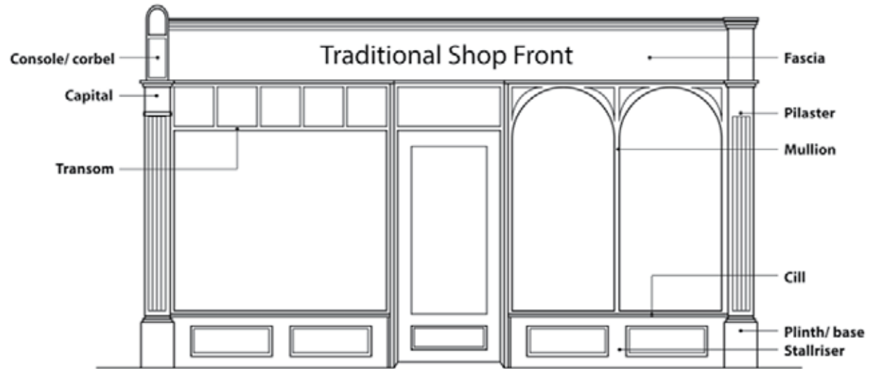
The components of a traditional shop front
